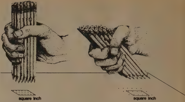
Energy density is determined by the angle of incidence.
